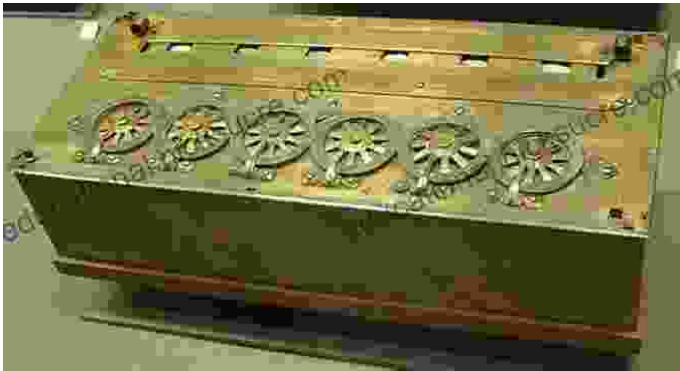
In the 17th century, French philosopher and mathematician Blaise Pascal invented the Pascaline, the first mechanical calculator. This groundbreaking device used a series of gears and levers to perform addition and subtraction automatically. The Pascaline revolutionized the field of mathematics, making it possible to perform complex calculations with greater speed and accuracy.
